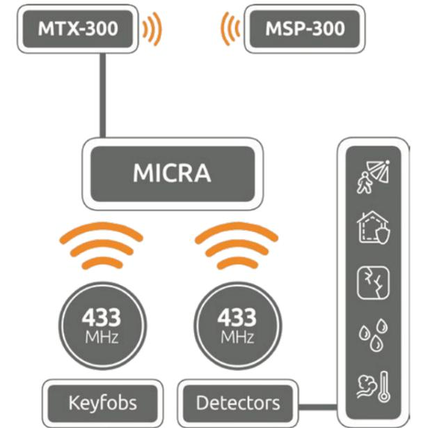
The MTX-300 can also be connected to the MICRA module to extend its functionality by adding capability to control the MSP-300 wireless sirens. Wired inputs of the module can be used to receive signals from an increased number of detectors. As a result, the MTX-300 makes it possible to use up to 12 wireless detectors in the system or expand it by adding extra keyfobs.
