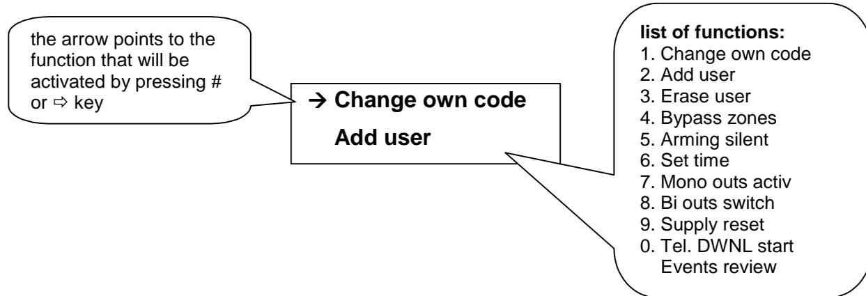
The ▲ and ▼ keys enable scrolling through the user functions. [#] and ► keys activate the given function. It is possible to activate a function directly - when User Functions Menu appears
