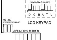
Only zone expanders with version 2 are allowed (label dated February 1998 or later). Since LCD keypads take larger current then LED keypads (especially when backlighting is on), wire resistance must be taken into account in the case of supply and earth cables.
