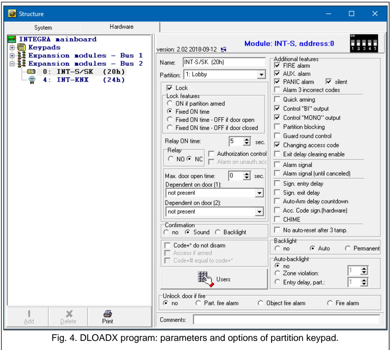
Fig. 4. DLOADX program: parameters and options of partition keypad.
