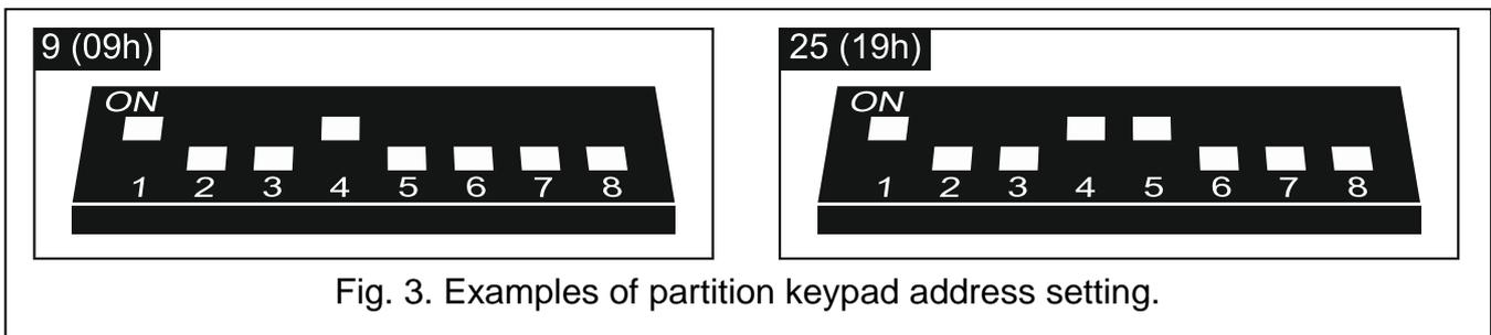
Fig. 3. Examples of partition keypad address setting.
