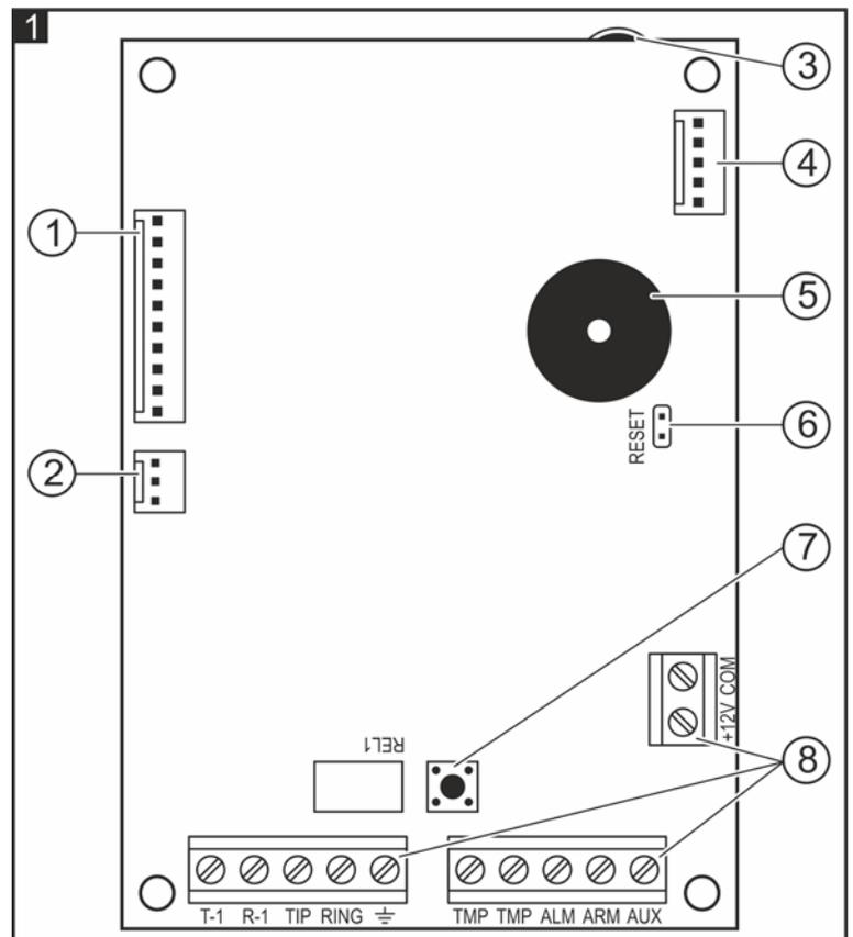
**T-1; R-1** - telephone line output (telephone set connection).
