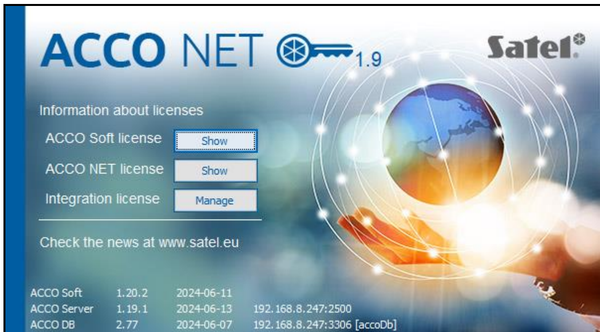
Fig. 4. Window with information on versions of ACCO NET system, programs and database, and with license access buttons.
