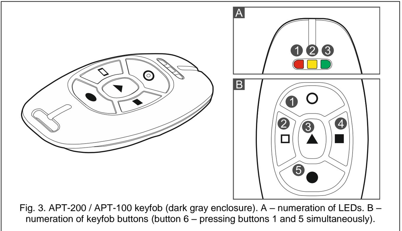
Fig. 3. APT-200 / APT-100 keyfob (dark gray enclosure). A – numeration of LEDs. B – numeration of keyfob buttons (button 6 – pressing buttons 1 and 5 simultaneously).
