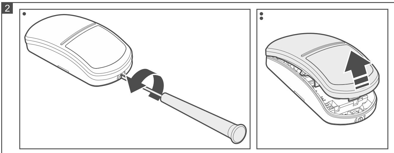
2. Press the catches and move the electronics module down, then remove it from the enclosure base (Fig. 3).
