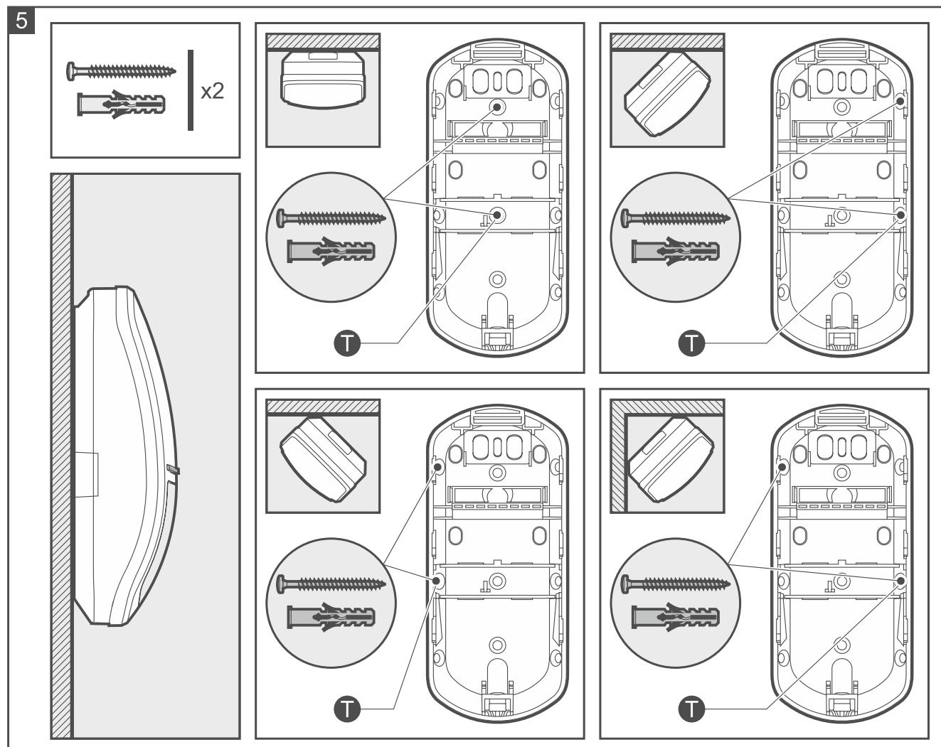
4. If the detector is to be secured to the wall with screws (Fig. 5) or to a bracket mounted on the wall or ceiling (Fig. 6):
