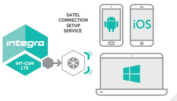
Communication with the control panel via the **INT-GSM LTE** module can take place through the SATEL connection setup service.
