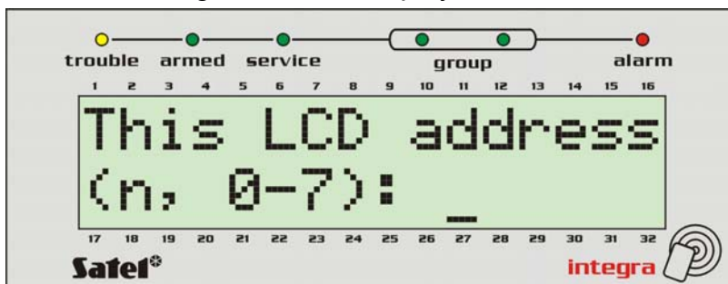
Fig. 18. Programming the keypad address
